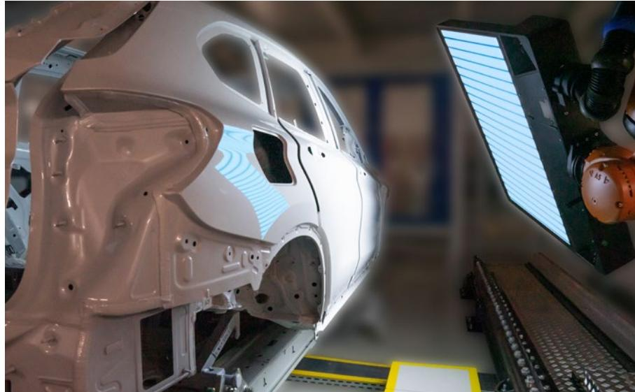
By combining surfaceCONTROL in the body shop and reflectCONTROL in the paint shop, Micro-Epsilon provides a comprehensive inspection concept that covers the entire car body manufacturing process. The results from both systems can be superimposed to ensure consistent quality assessment throughout the entire manufacturing process. Therefore, car manufacturers benefit from high measurement accuracy, reliable processes, and a significant improvement in the overall quality of the car body.
